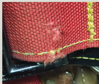
Broken webbing strands show up as tufts on webbing surface.
