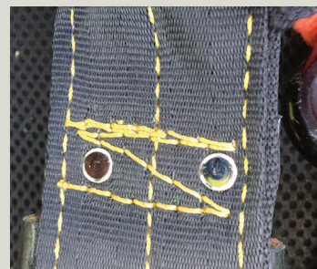
Closely inspect the box stitches; these are the strong points in the saddle and if several strands are broken, saddle must be taken out of service.
