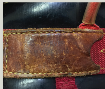
Life of saddle is five years. If no longer able to determine issue date, remove from service.
