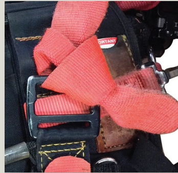
Ensure friction buckles are not broken or missing - photo of saddle has missing buckle and trimmer simply tied a knot!
