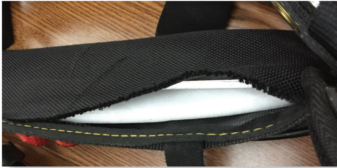
Stitching in Battan Seat is torn. If any of the white material underneath the black outer coating is visible, immediately remove the equipment from use.
