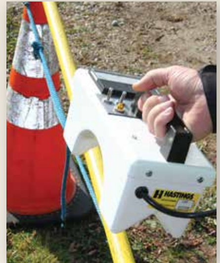
Regional safety personnel have begun field testing pruner poles to determine which poles will be considered non-conductive tools approved for use within (MAD).
